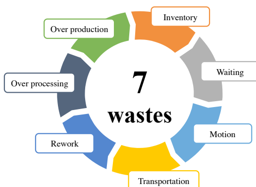
Figure 3-6: Seven waste around our working environment
